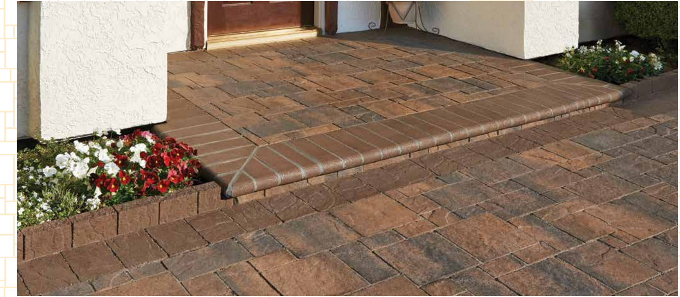
Above: Cream-Brown-Charcoal Heartland Paver installed in a random ashlar pattern. Step is solid Mocha Bullnose coping. The border and edger is solid mocha Slate Stone 'B' 6x9 (distressed). The edger was field-split to achieve the top texture.
